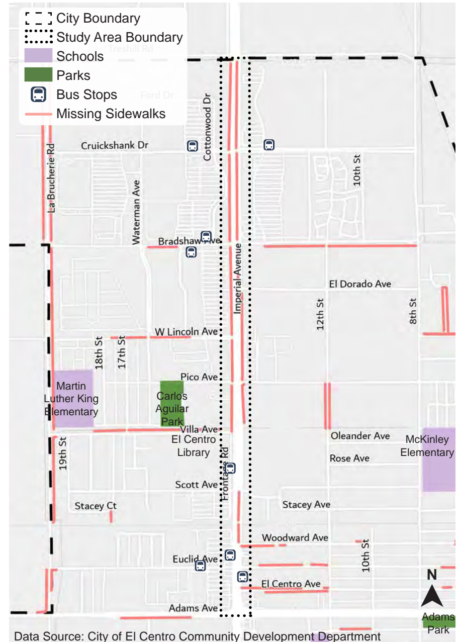
Figure 2-4: Missing Sidewalks on Imperial Avenue
